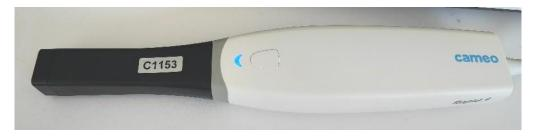
Step 5: Finish the calibration and remove calibration tip.
