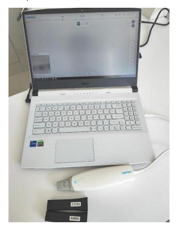
Step 2: Click " on the main interface to enter the calibration interface. Click the calibration button. Calibration begins.
